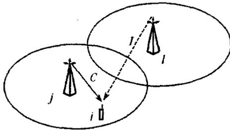
Figure 2. Link between mobile station  $i$  and base station  $j$  and interference of the base station
